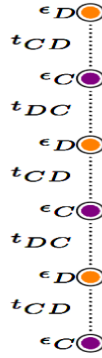
Figure 7.2: One-dimensional free-free di-atomic lattice, ( \epsilon_k = \epsilon_C, \forall odd k , \epsilon_k = \epsilon_D, \forall even k , t_k = t_{CD}, \forall odd k , t_k = t_{DC}, \forall even k )
