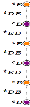
Figure 7.5: One-dimensional free-free di-atomic lattice, ( \epsilon_k = \epsilon_D, \forall odd k , \epsilon_k = \epsilon_E, \forall even k , t_k = t_{DE}, \forall odd k , t_k = t_{ED}, \forall even k )
